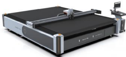
LC8-3225 Large format cutting Working Range: 3200*2500mm Product Size: 3950*3560*1221mm
