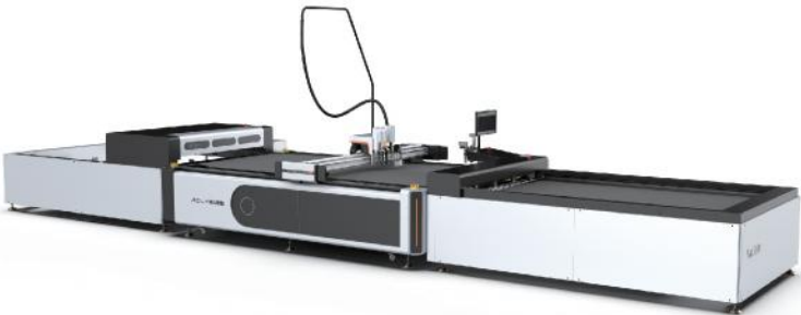
LC8-1625 Loading and unloading system Working Range: 1600*2500mm Product Size: 10660*2620*1280mm
