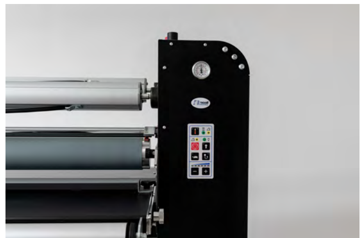
Interface and pneumatic control
