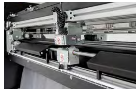
Self sharpening pneumatic vertical cutters
